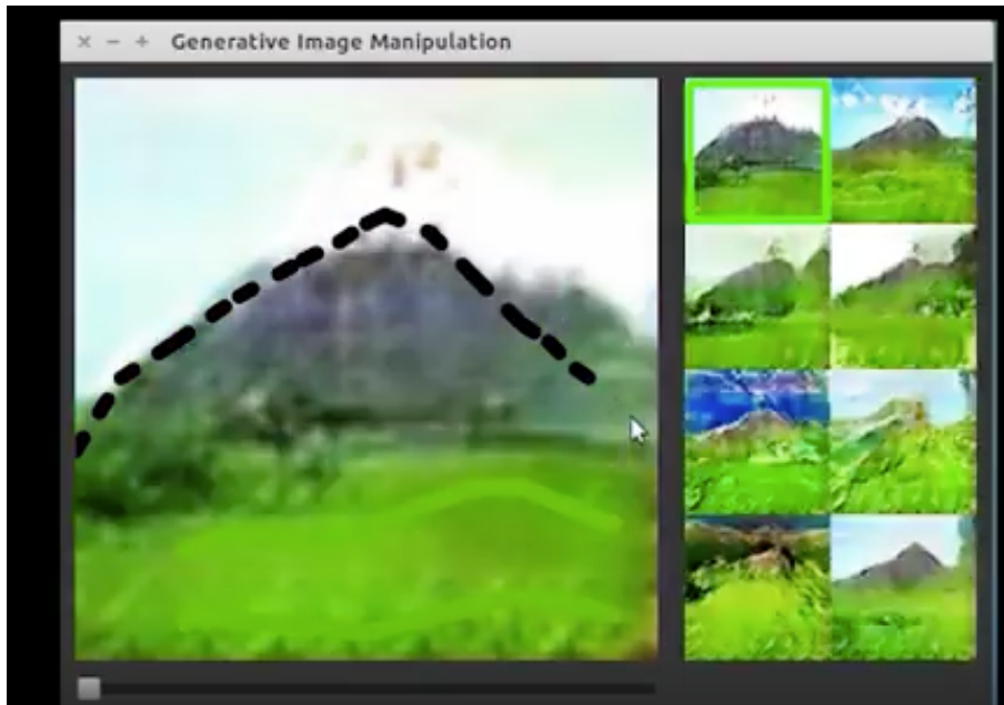
Figure 5: Zhu et al. (2016) developed an interactive application called interactive generative adversarial networks (iGAN). A user can draw a rough sketch of an image, and iGAN uses a GAN to produce the most similar realistic image. In this example, a user has scribbled a few green lines that iGAN has converted into a grassy field, and the user has drawn a black triangle that iGAN has turned into a detailed mountain. Applications that create art are one of many reasons to study generative models that create images. A video demonstration of iGAN is available at the following URL: https://www.youtube.com/watch?v=9c4z6YsBGQ0
